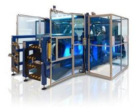
The completely automatic dual coiler TR1400, by FB Balzanelli, is designed to coil flexible PE and XPE-AI-XPE pipes and copper tubing with diameters ranging from 10 to 50 mm. Each unit is automatically adjusted thanks to sophisticated software that makes it possible to program the management of different production lots and achieve precision pipe cutting on point zero. The technology developed by FB Balzanelli also reduces pipe ovalization during winding.
